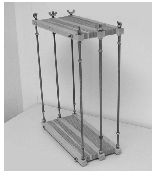
Figure 6 Etching tool capable of holding 20 boards (300 x 450 mm) at one time
